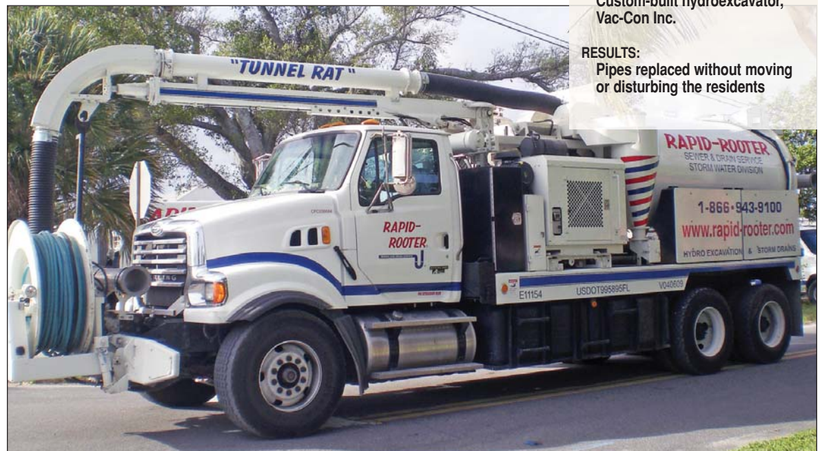
Top: Workers shovel clean mason sand into the gunite hopper during the backfilling process. Right: Rapid-Rooter's Vac-Con hydroexcavator was custom built by Southern Sewer Equipment Sales, Ft. Pierce, Fla. (Photos courtesy of Rapid-Rooter Plumbing Sewer & Drain Services)
